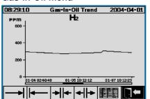
Individual chart diagram for hydrogen H<sub>2</sub>, carbon monoxide CO and moisture-in-oil (H<sub>2</sub>O in ppm and %)
