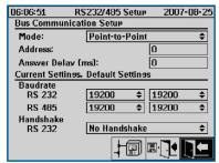
Transmission speed adjustment for the RS 232 / RS 485 connection
