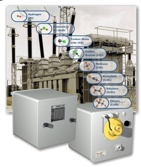
The HYDROCAL 1008 is a permanently-installed multi-gas-in-oil analysis system with transformer monitoring functions. It allows for the individual measurement of moisture and the key gases hydrogen (H<sub>2</sub>), carbon monoxide (CO), carbon dioxide (CO<sub>2</sub>), methane  $(CH_4)$ , acetylene  $(C_2H_2)$ , ethylene  $(C_2H_4)$  and ethane (C<sub>2</sub>H<sub>6</sub>) dissolved in transformer oil.
