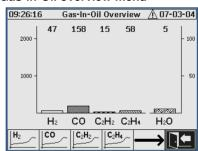
Individual chart diagram for hydrogen (H<sub>2</sub>), carbon monoxide (CO), carbon dioxide  $(CO_2)$ , methane  $(CH_4)$ , acetylene  $(C_2H_2)$ , ethylene (C<sub>2</sub>H<sub>4</sub>) and ethane (C<sub>2</sub>H<sub>6</sub>) and moisture.
