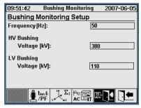
The bushing monitoring setup menu allows the input of all basic parameters required for the bushing monitoring.
