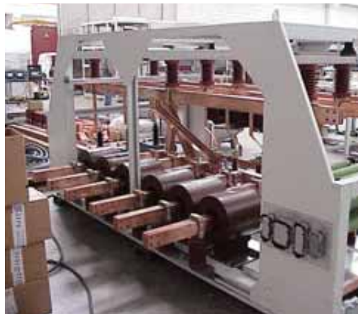
> AGN-24 Transformer for generator switchgear.
